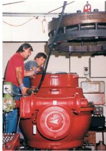
Final inspection (pressure testing) of a KLINGER Ballostar KHSVI ball valve acc. to DIN 3230
