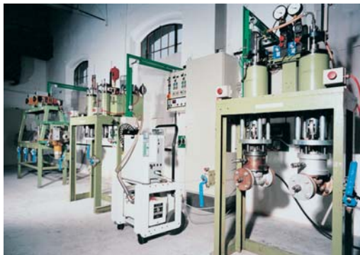
KVN KX1-GT 50.000 cycle test
